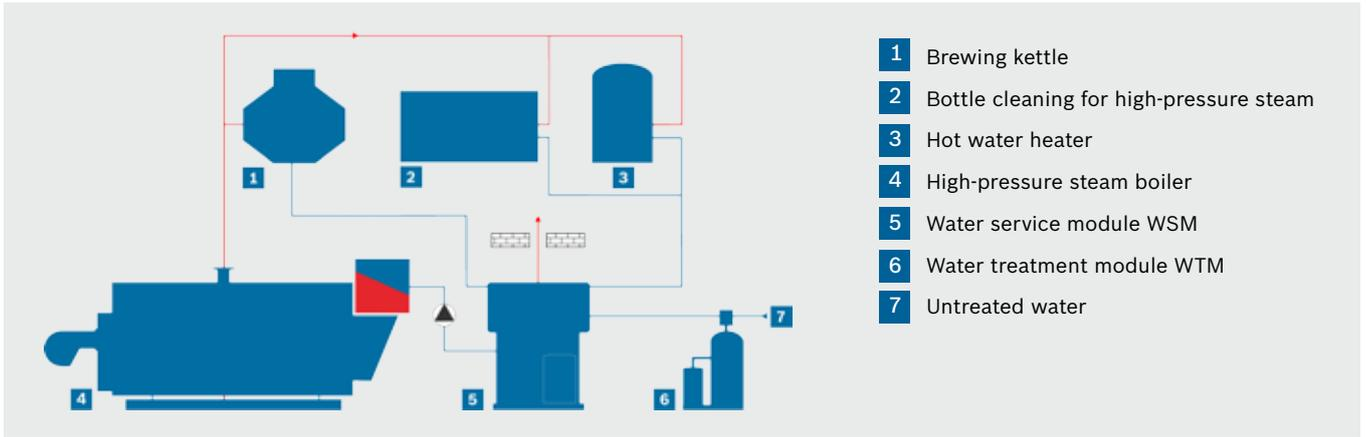
Figure 1: Steam generation for a restaurant brewery with open condensate recirculation
