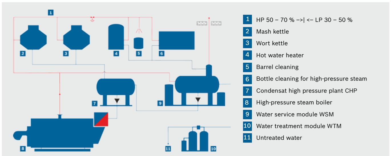
Figure 3: Concept for a partial renewal and use of a HP condensate service module
