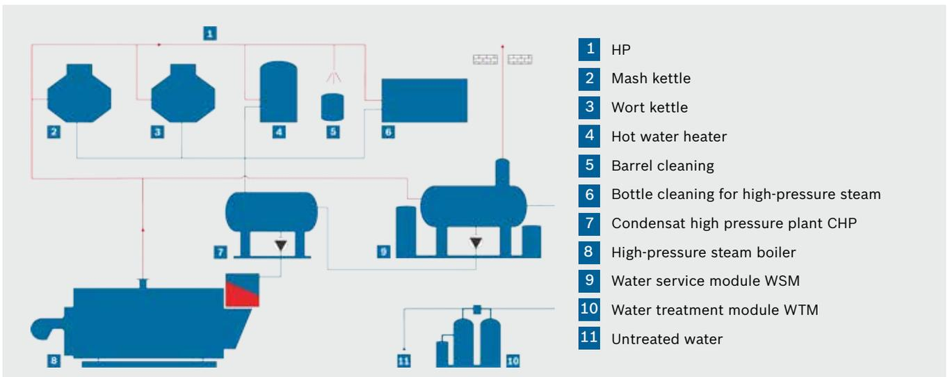
Figure 2: New construction of a steam generating concept for medium-sized and large breweries with closed condensate recirculation
