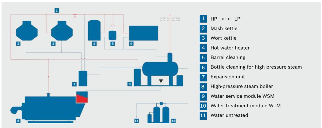
Figure 4: Concepts with partial deaeration using a low-priced expansion unit
