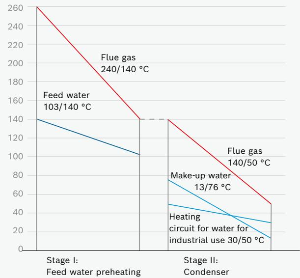
Figure 6: Two-stage flue gas heat recovery with flue gas/water temperature at 100% load.
