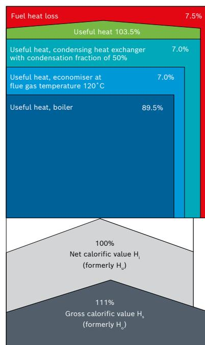
Figure 9: Heat balance of a steam generator with condensing technology.
