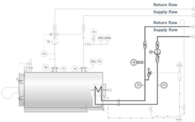
Figure 5: Hydraulic circuit for optimal use of condensing technology.
