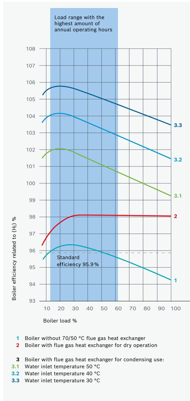
Figure 2: Efficiency curves for condensing technology (using a hot water boiler with gas combustion as an example).
