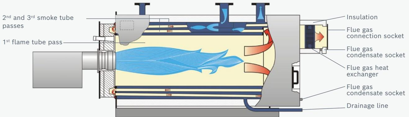
Figure 3: Cross-section of a Bosch heating boiler (UT-L) with an integrated flue gas heat exchanger.
