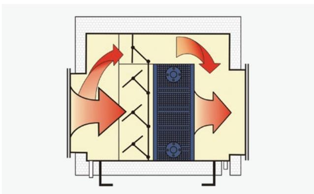
Figure 4: Flue gas heat exchanger for separate installation and retrofitting.
