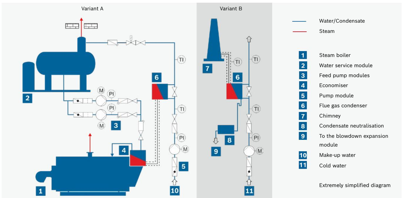
Figure 7: Simplified diagram of a high-pressure boiler system with two flue gas heat exchanger stages (economiser/flue gas condenser).
