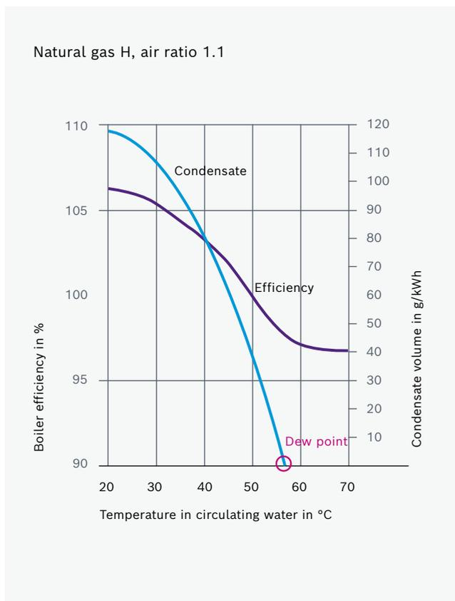
Figure 1: Influence of the circulating water temperature on the boiler efficiency and the condensate accumulation rate for natural gas.
