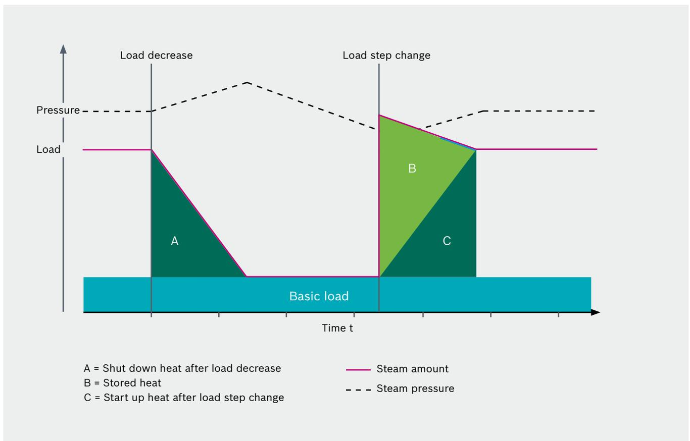
Graphic: Steam parameters at paper break – every paper break is quickly controlled
