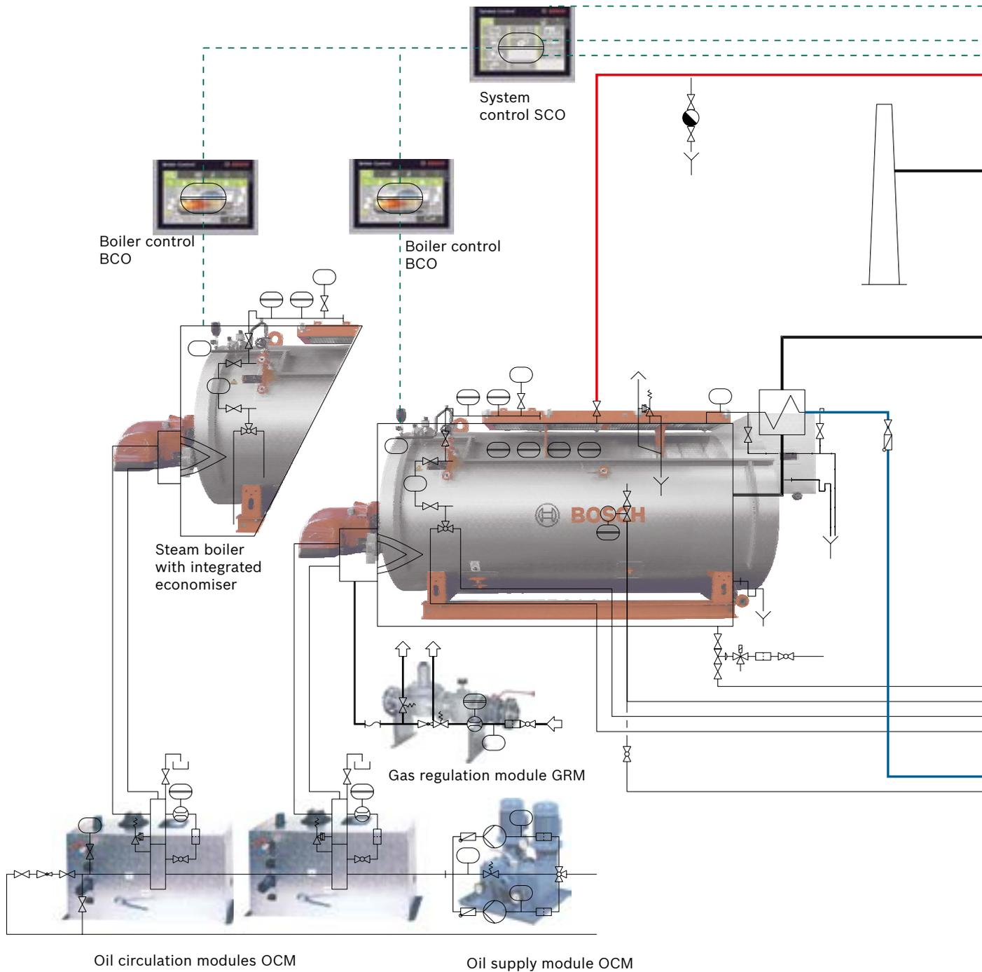
**Fig. 196** Function diagram of boiler house components
