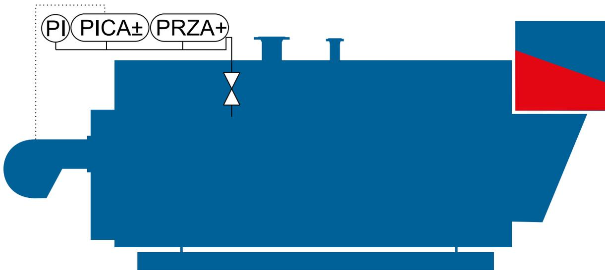
**Fig. 64** Heat maintenance via the combustion system
