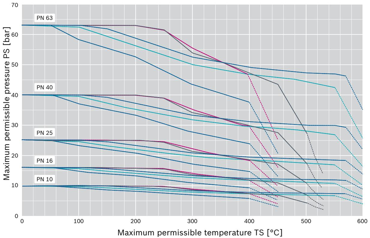
**Fig. 119** Pressure-temperature assignment for flanges according to EN 1092-1
