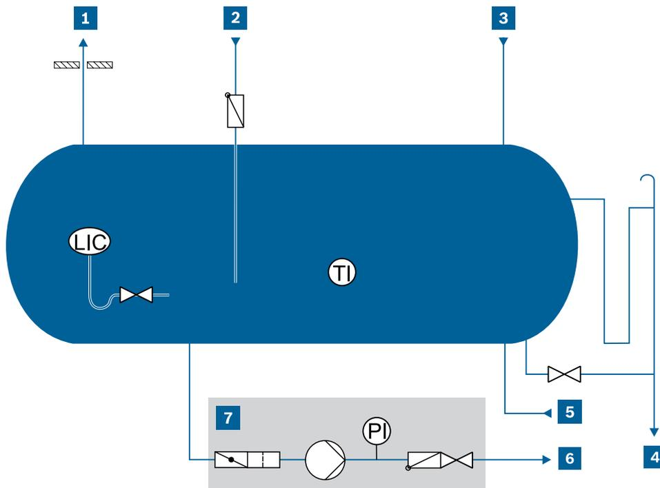
**Fig. 111** Schematic diagram of condensate tank – low pressure
