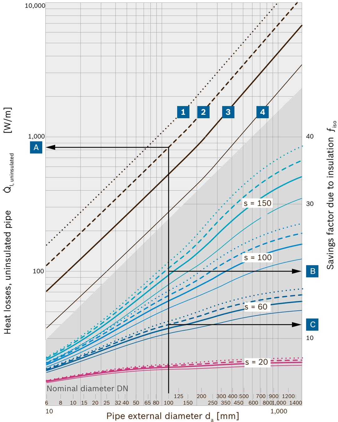
**Fig. 163** Savings factor due to insulation and heat losses in pipework
