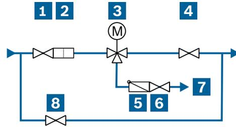
**Fig. 80** Feed water control module
