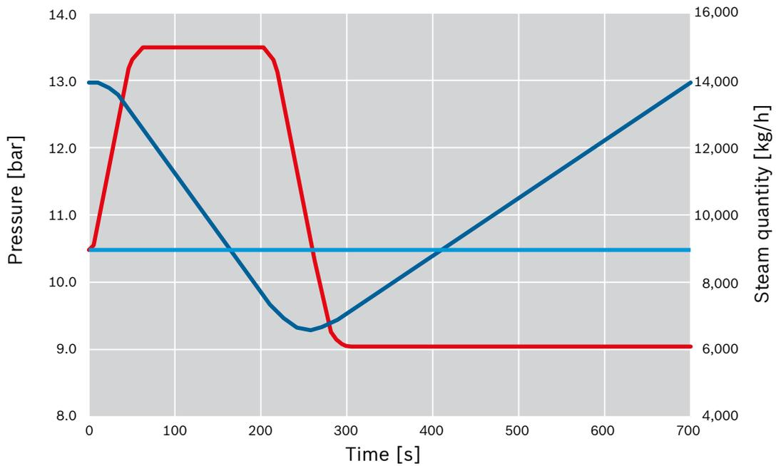
**Fig. 109** Pressure progression in a steam accumulator (example 1)
