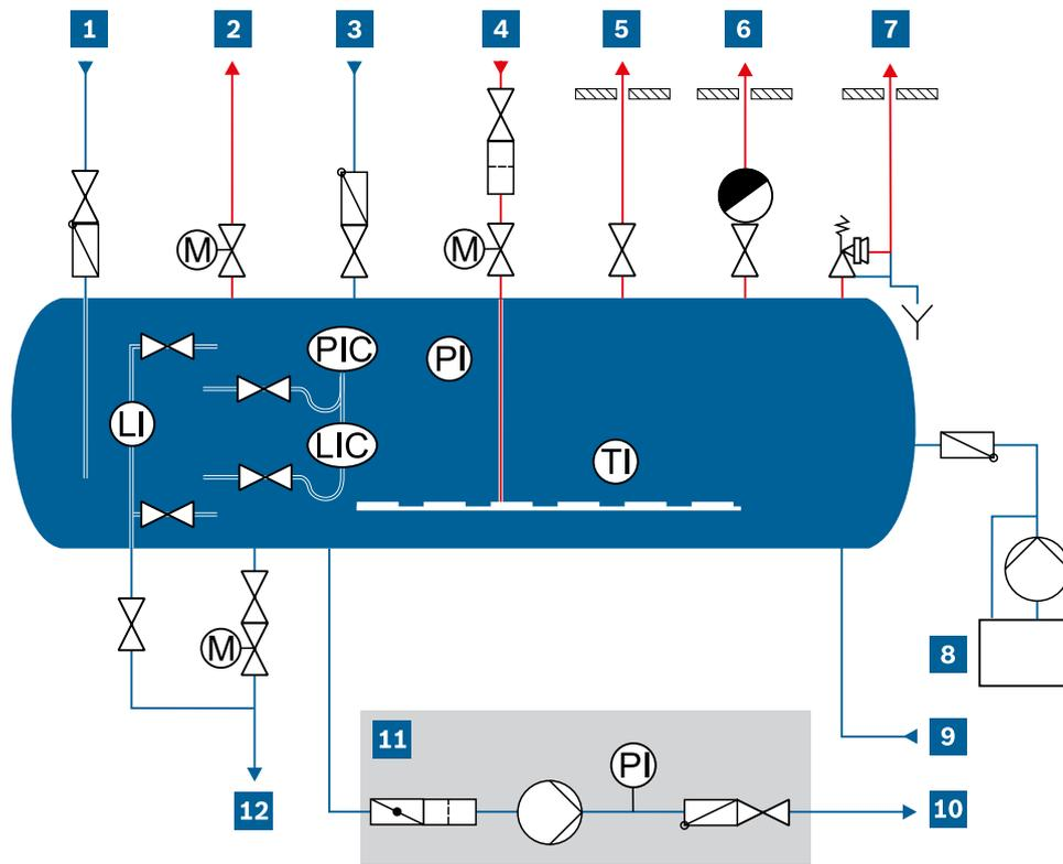
**Fig. 112** Schematic diagram of condensate tank – high-pressure
