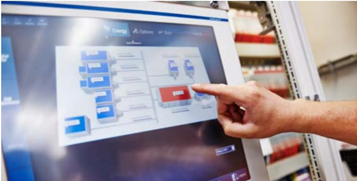
**Fig. 226** MEC System for coloured clear visualisation of location and operating conditions, temperatures and performance of systems
