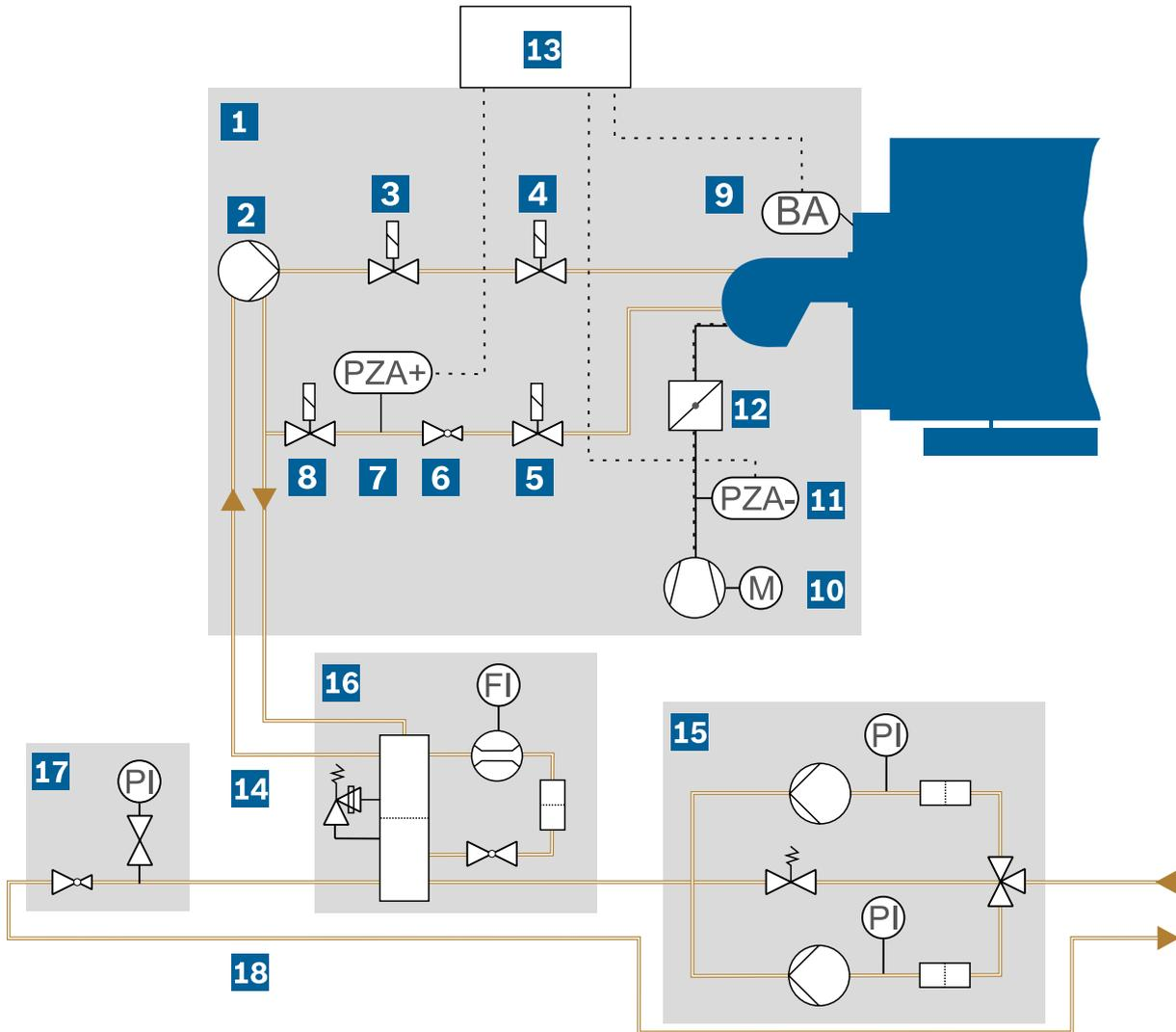
**Fig. 52** Example of a light fuel oil combustion system with pressure-jet oil burner
