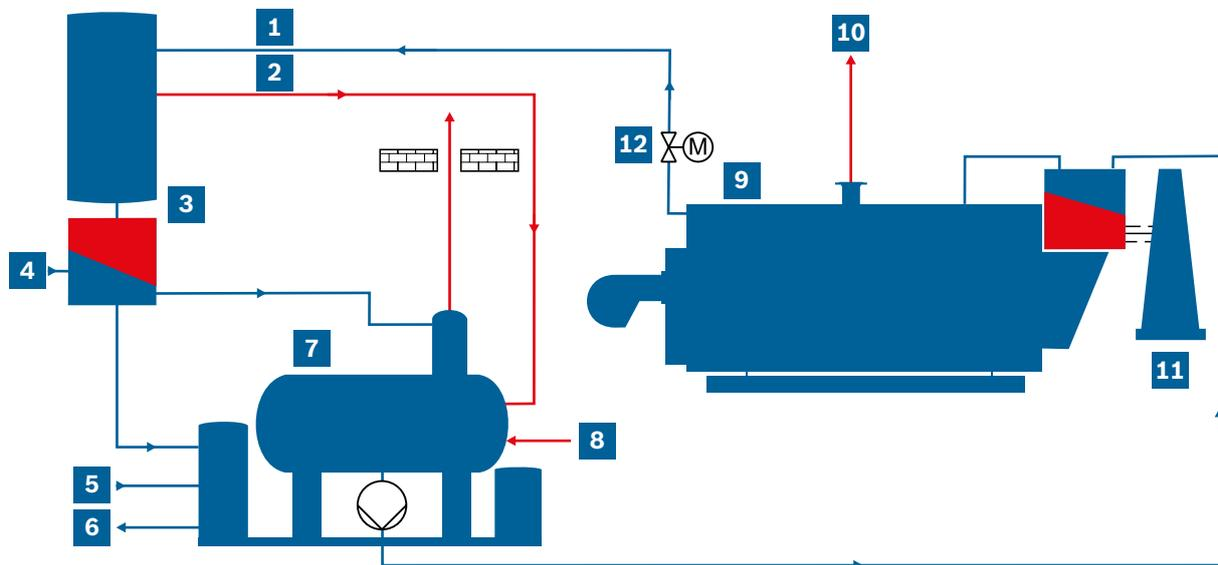
**Fig. 156** Schematic representation of expansion and heat recovery
