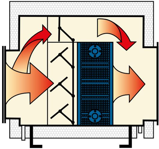
**Fig. 68** Condensing heat exchanger
