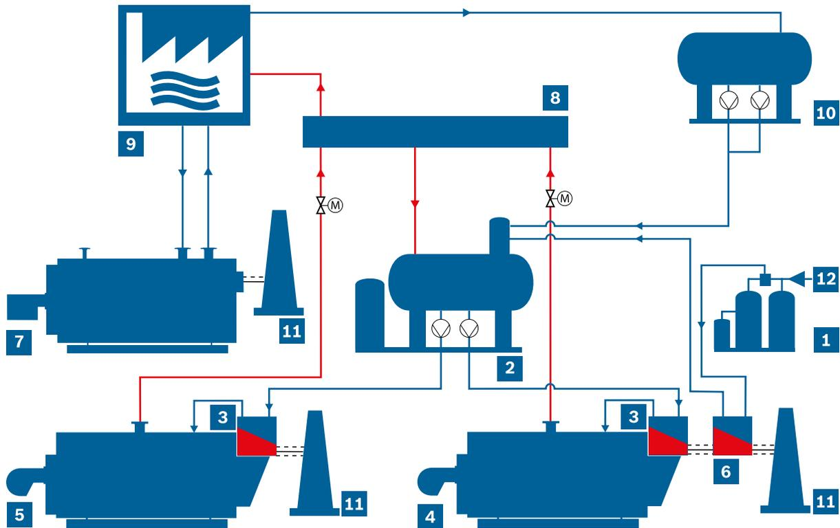
Fig. 160 Schematic representation of an open condensate system
