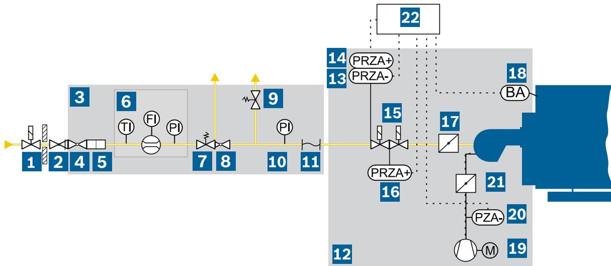
Fig. 59 Example showing schematic representation of gas combustion (high-pressure supply)
