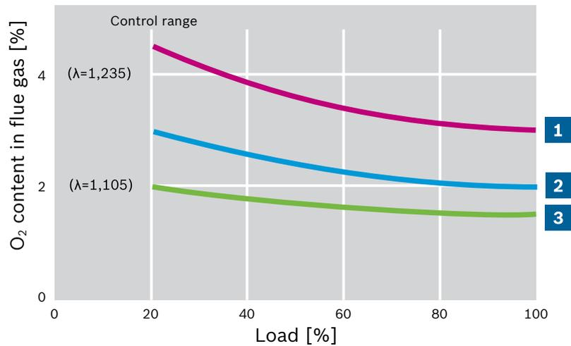
**Fig. 153** Residual oxygen content and excess air using O<sub>2</sub> and CO control via the burner load
