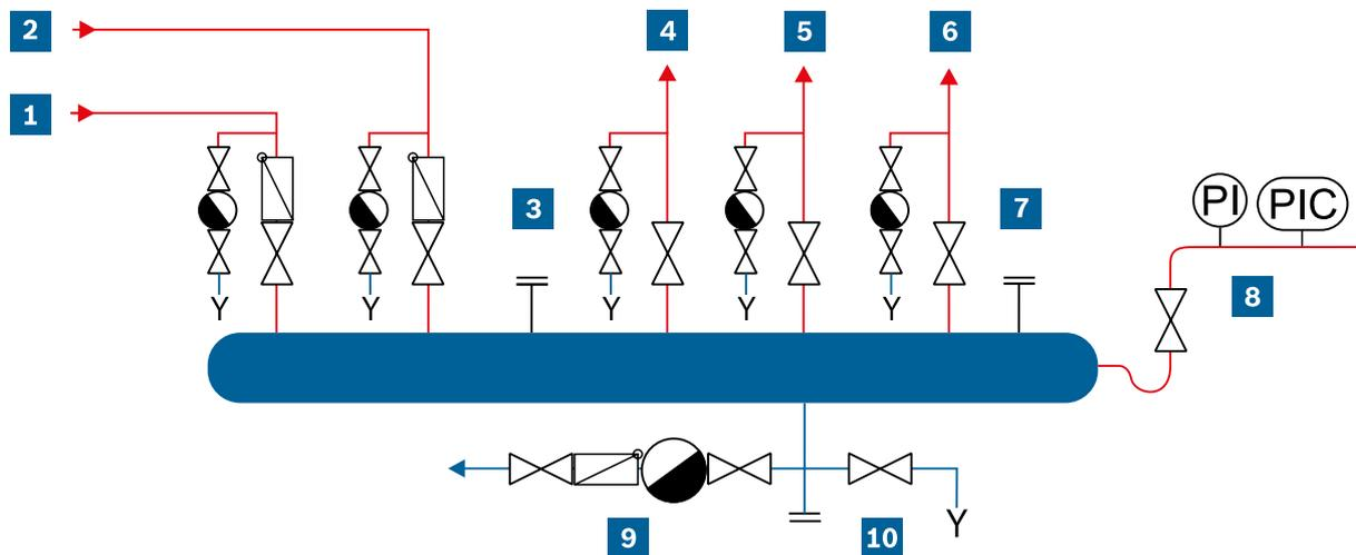
Fig. 105 Schematic representation of a steam distributor
