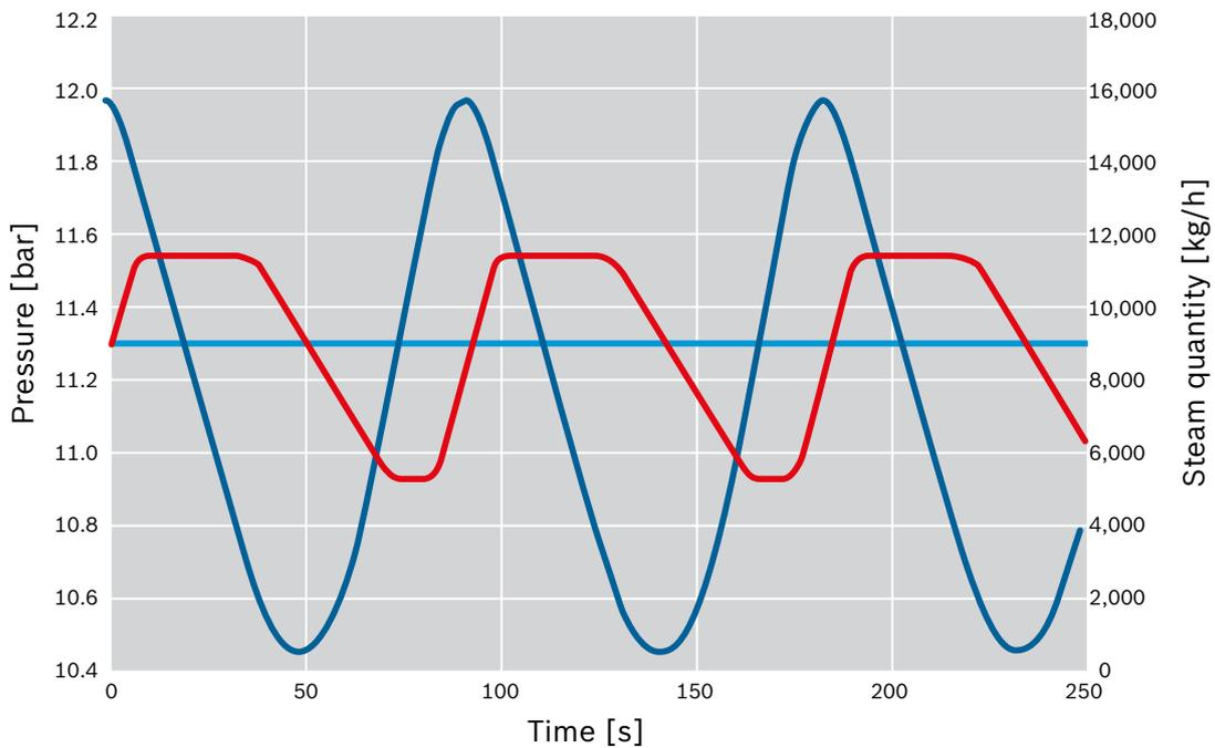
**Fig. 110** Pressure progression in a steam accumulator (example 2)
