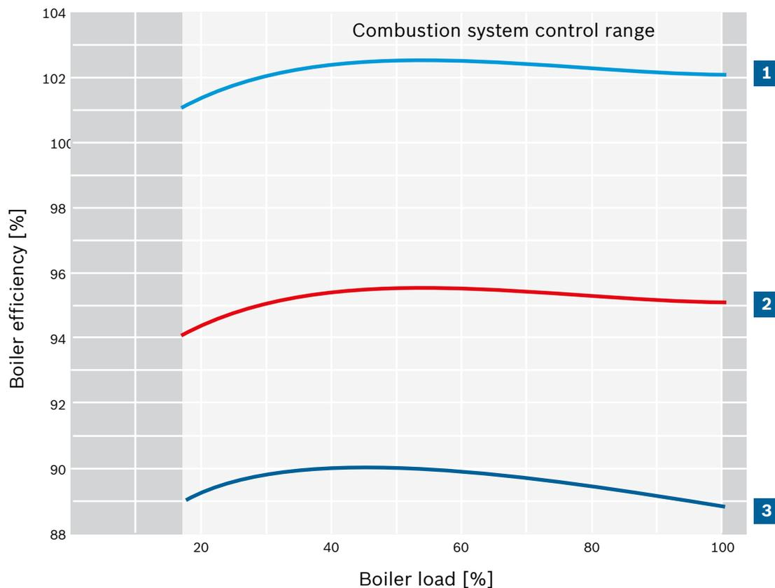
**Fig. 144** Efficiency curve as a function of the boiler load of a boiler without economiser, boiler with economiser and boiler with economiser and additional condensing heat exchanger
