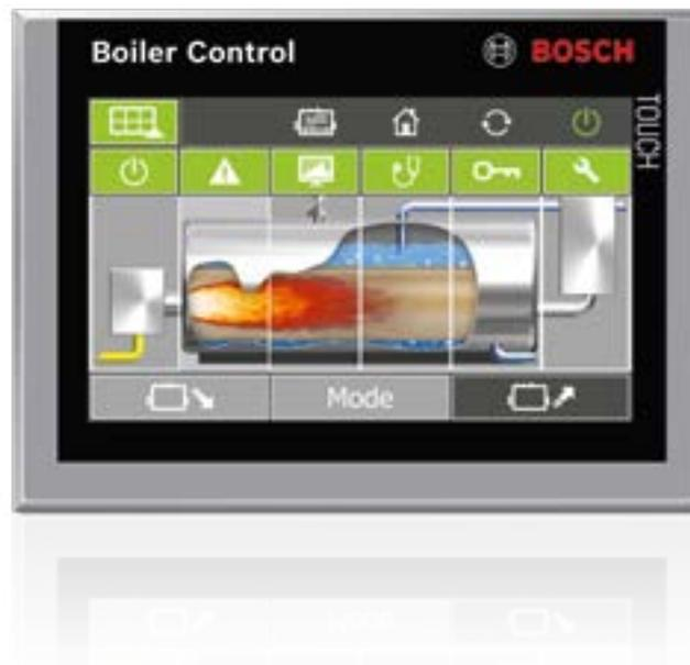
**Fig. 222** Home screen of boiler control BCO for steam boiler systems
