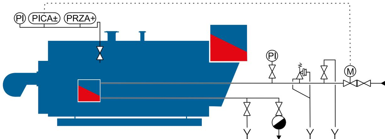
**Fig. 63** Heat maintenance via a heating coil
