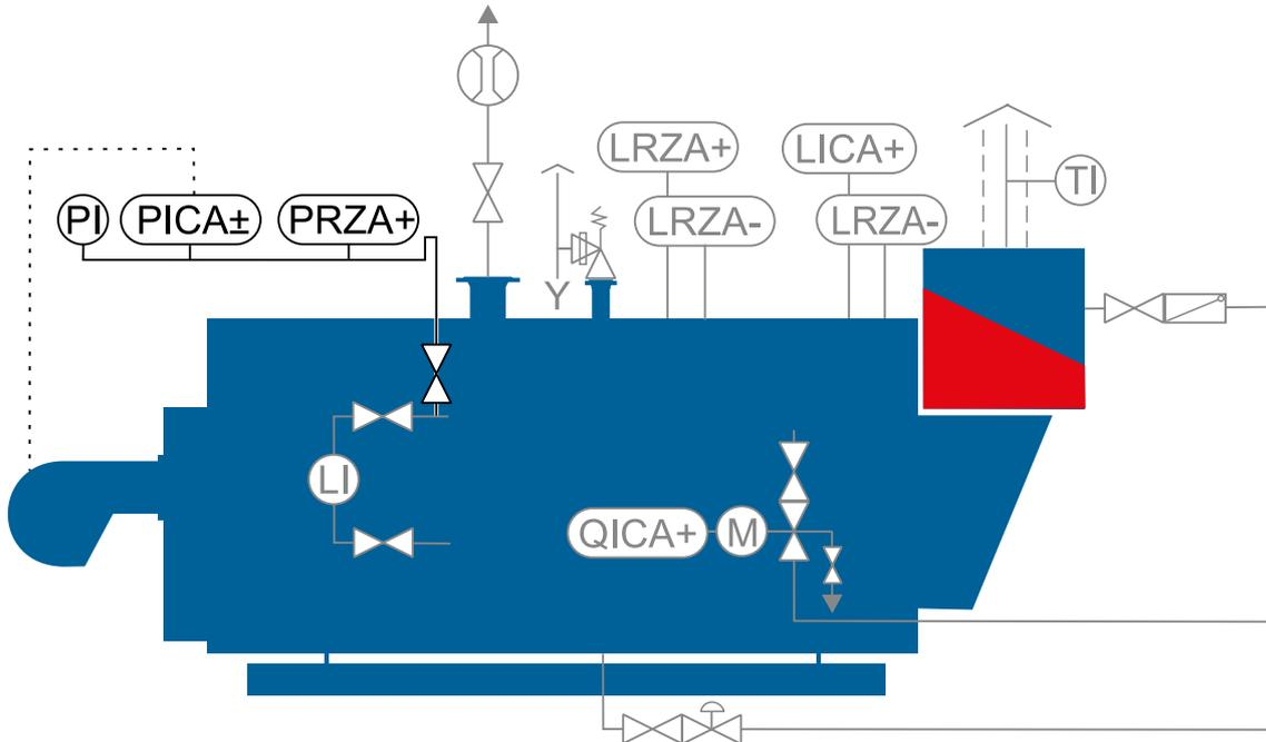
**Fig. 45** Pressure-controlled output control of a steam boiler
