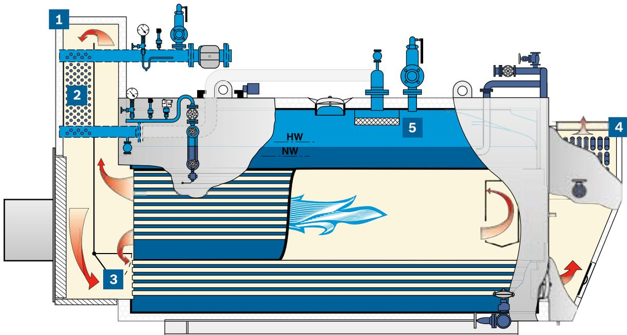
**Fig. 75** UL-S with mounted super heater
