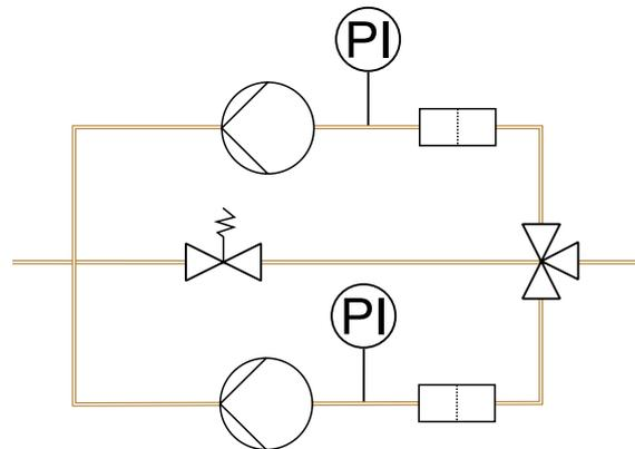
**Fig. 53** Oil supply module
