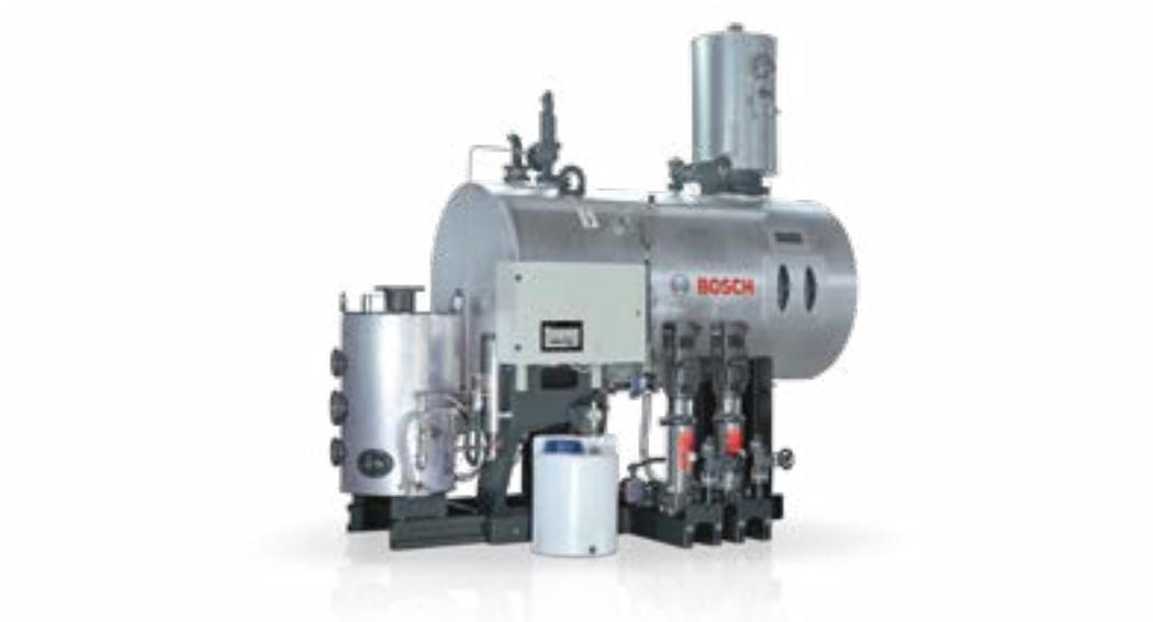
**Fig. 97** A water service module, consisting of feed water vessel with trickle deaerator, feed pump modules, blowdown expansion vessel, dosing tanks and corresponding control cabinet
