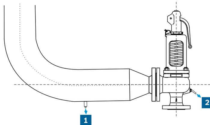
**Fig. 123** Drainage of blow-off pipe and safety valve
