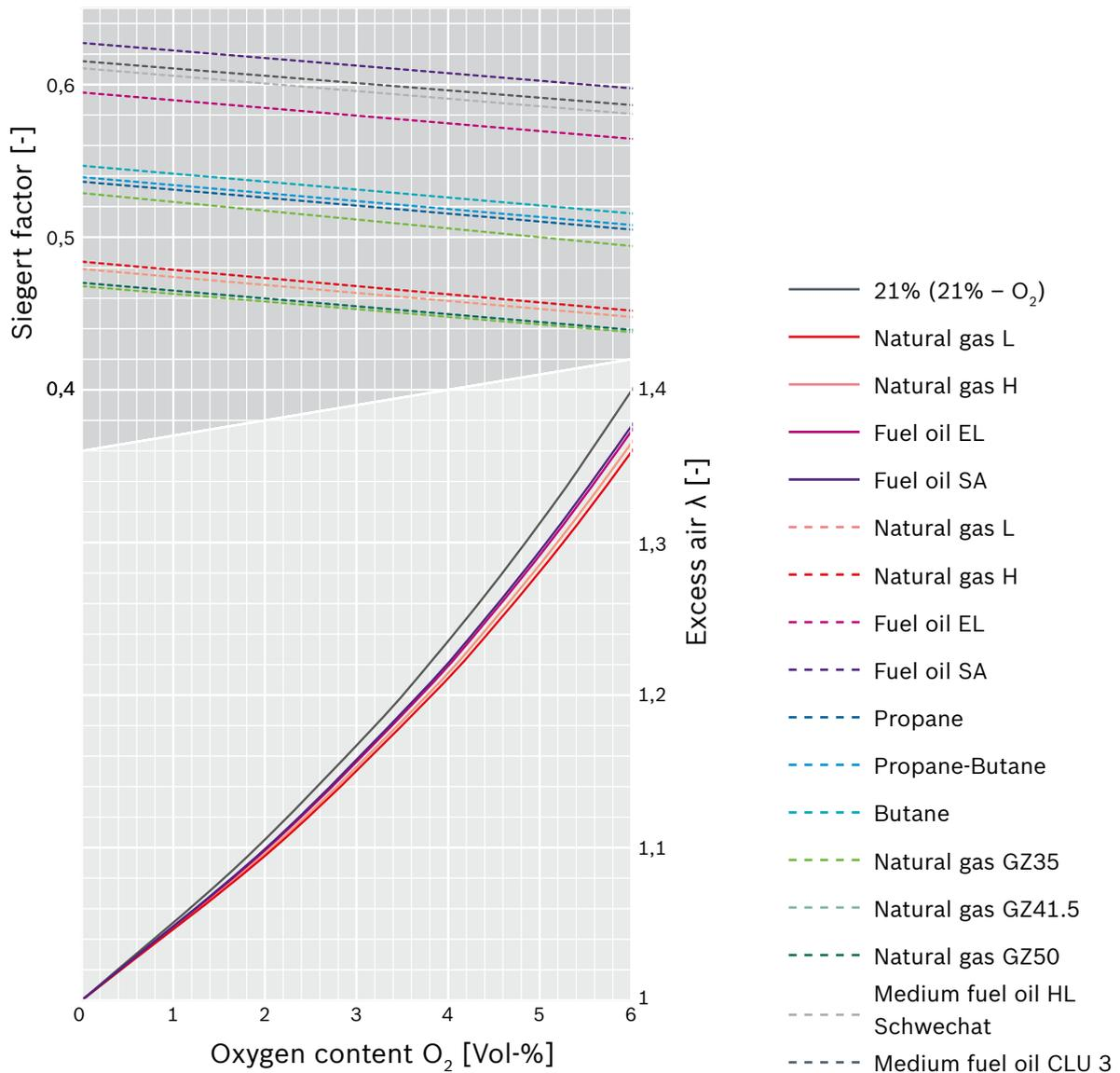
**Fig. 135** Correlation between oxygen content in dry flue gas, excess air and Sievert factor
