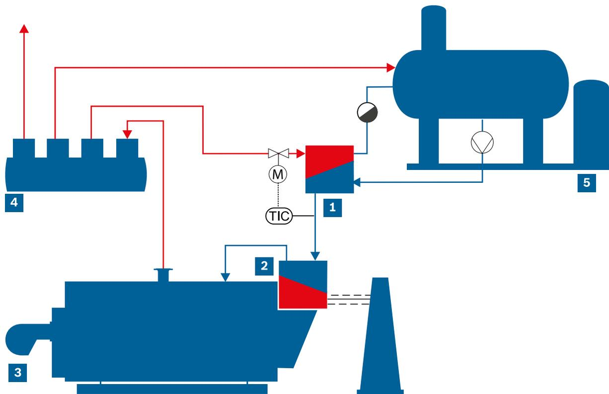
Fig. 72 Simplified system schematics showing integration of a feed water preheater
