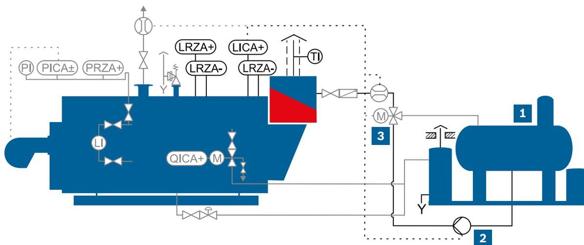
**Fig. 46** Level control of a steam boiler
