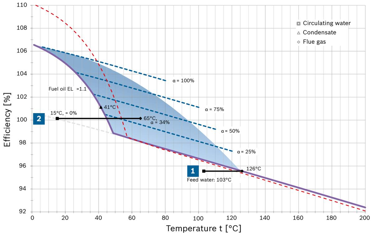
**Fig. 231** Pinch-point diagram for oil
