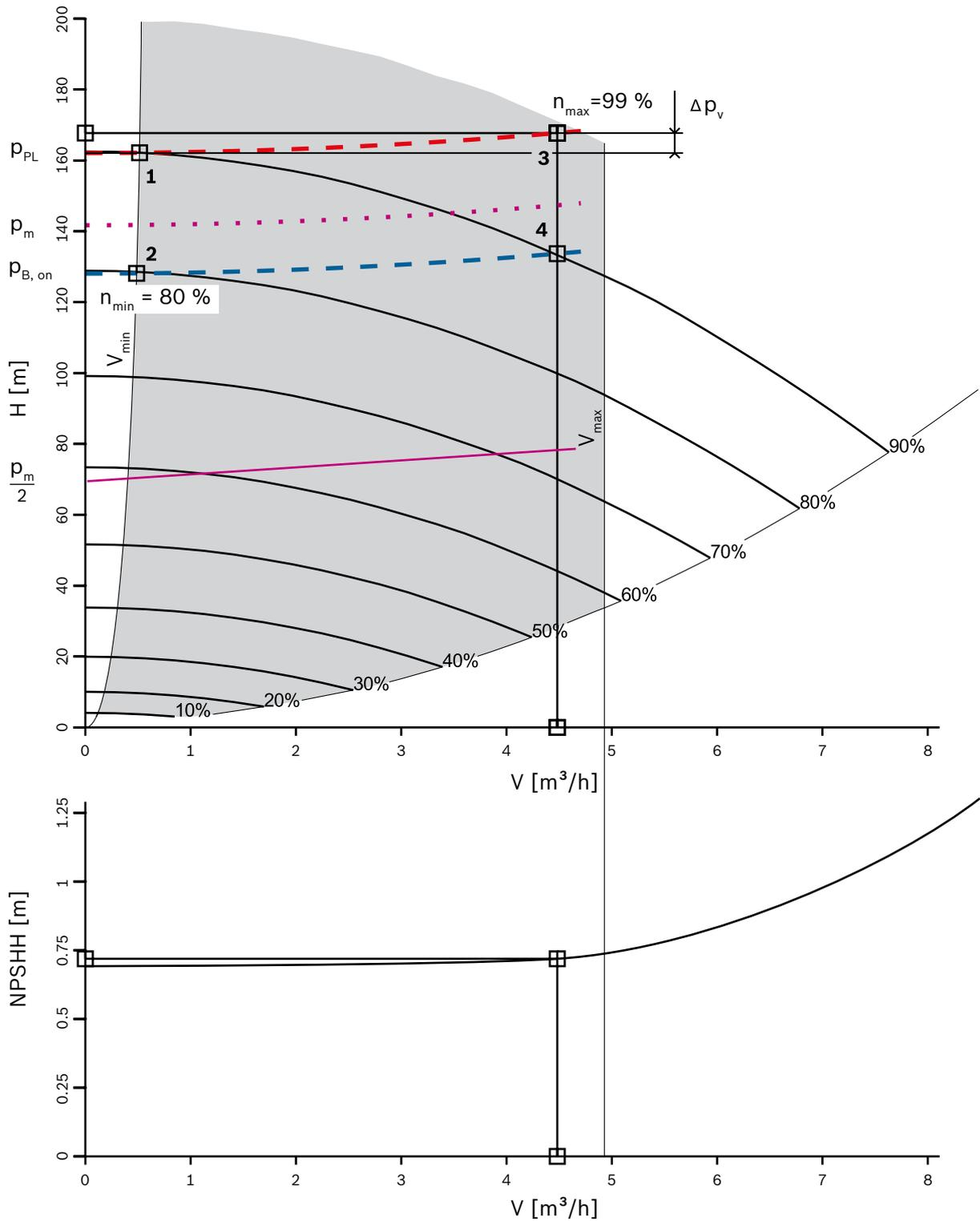
**Fig. 76** Example of a characteristic map of a speed-controlled boiler feed pump
