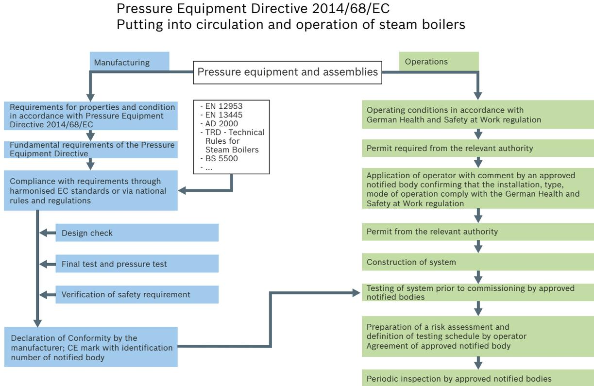
**Fig. 12** Procedure for manufacturing and operation based on the Pressure Equipment Directive 2014/68/EU<sup>IV)</sup>
