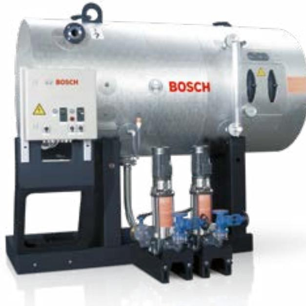
**Fig. 201** *The unpressurised condensate service module collects the condensate streams and channels them back into the water/steam circuit via the deaeration system*
