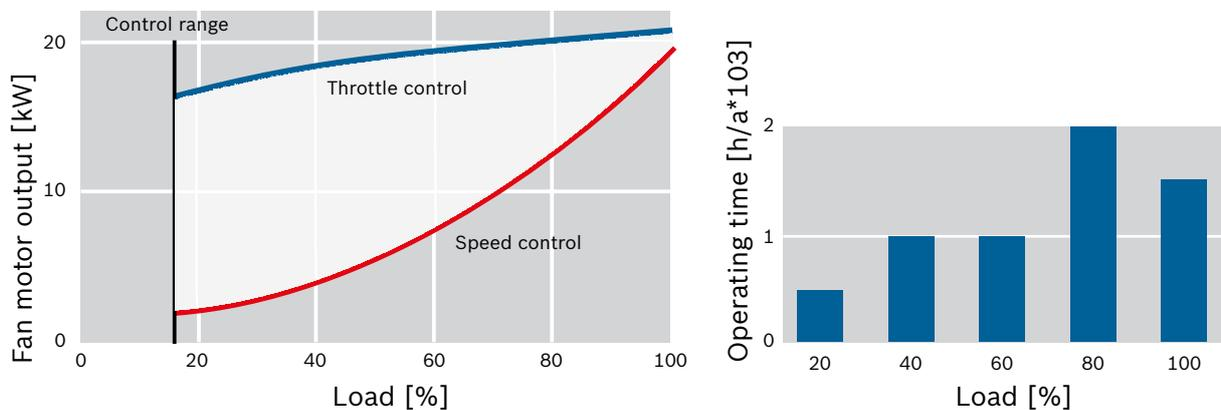
Fig. 151 Energy savings with speed-controlled burner fan
