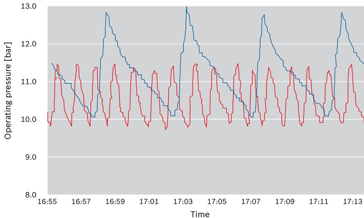
**Fig. 27** Reduction of burner cycling via optimised setting
