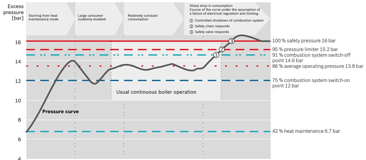
**Fig. 6** Diagram of pressure curve with switching points when using steam boilers with an average operating pressure of 13.3 bar
