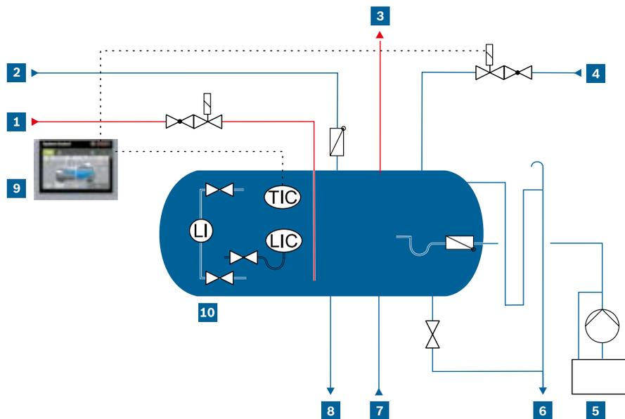
**Fig. 100** Feed water supply – partial deaeration
