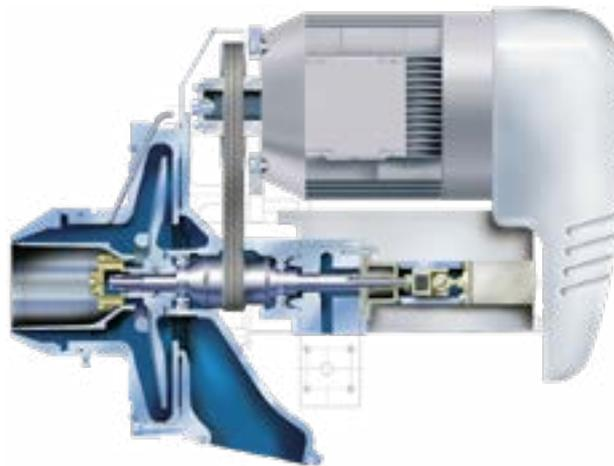
**Fig. 51** Sectional view of a rotary atomising burner (Saacke)
