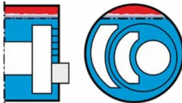
**Fig. 126** Boiler design with side-by-side arrangement of passes
