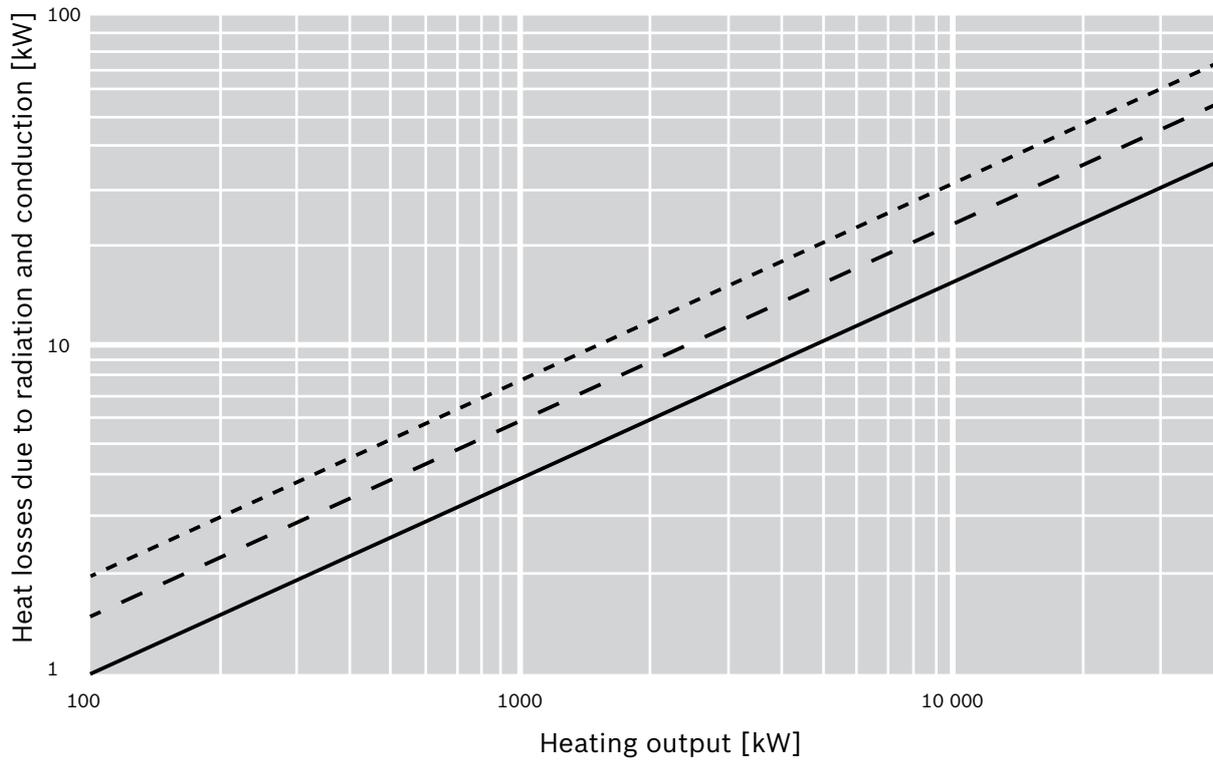
**Fig. 137** Heat losses due to radiation and conduction as a function of the nominal output of the boiler and of the average temperature of the medium in the boiler with an insulation thickness of 100mm
