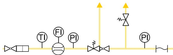
**Fig. 60** Gas regulation module
