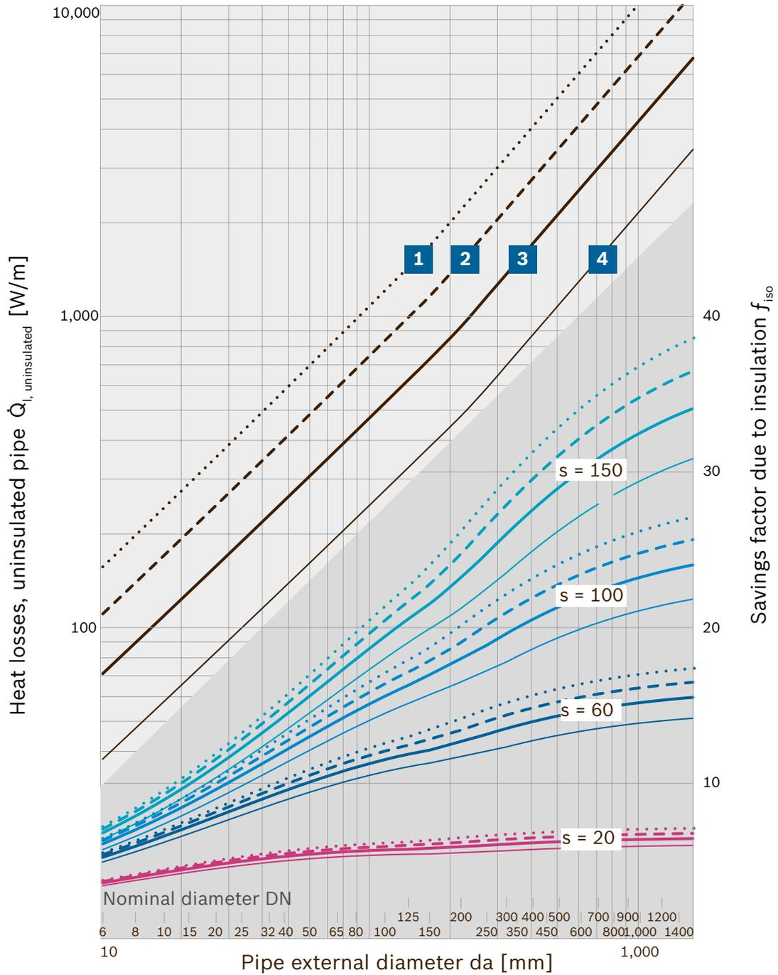
**Fig. 235** Savings factor due to insulation and heat losses in pipework
