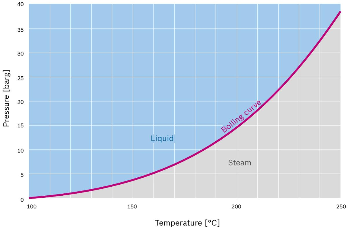
**Fig. 37** Boiling curve of pure water in pressure-temperature graph (range < 40 bar)
