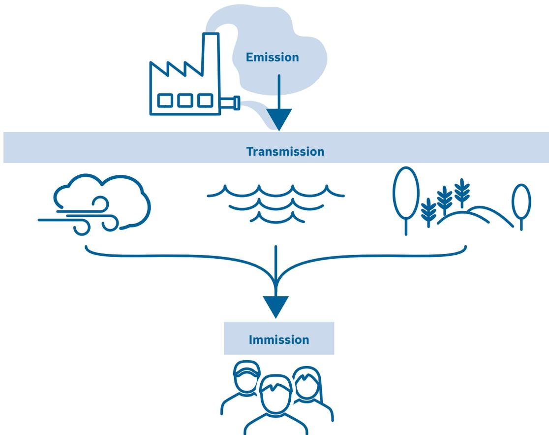
**Fig. 14** Difference between emission, transmission and immission
