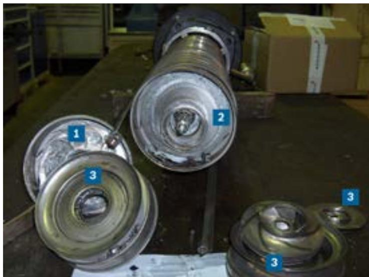
**Fig. 26** Pump damage due to cavitation
