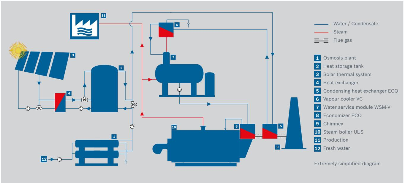
System diagram steam boiler combined with a solar thermal system and heat recovery modules.
