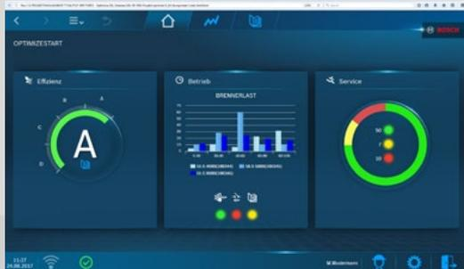
MEC Optimize captures all the operating parameters and messages of the linked system components. Over many years the data are stored locally, which means that the plant operator remains the data owner. The visualization takes place in the three separate areas of efficiency, operation and service and provides a comprehensive analysis.
