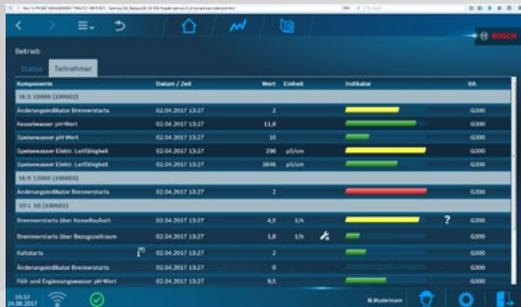
After an automated data analysis the system indicates any increased energy consumption as well as evaluates the system's operating performance. Based on their load profile components are assessed for wear which enables the plant operator to ensure that system availability is maintained.
