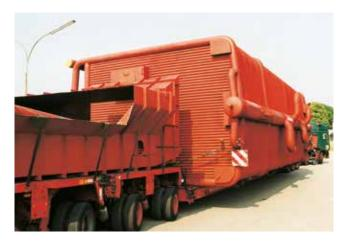
Figure 2: 100 MW hot water - water tube boiler during transport
