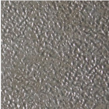
Figure 6: External cladding with a textured aluminium sheet
