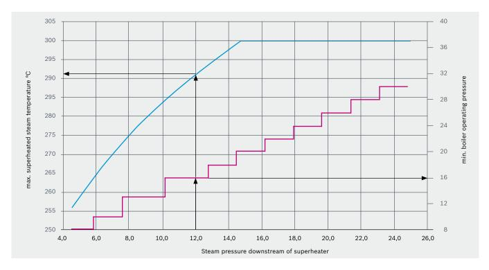
Graphic 1: The graphic shows the max. possible superheated steam temperatures and the min. required pressure stage depending on the requested steam pressure downstream of the superheater
