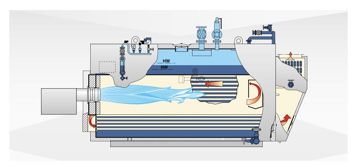
Figure 1: UNIVERSAL UL-S steam boiler with integrated Economiser
