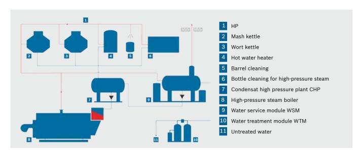
Figure 2: New construction of a steam generating concept for medium-sized and large breweries with closed condensate recirculation
