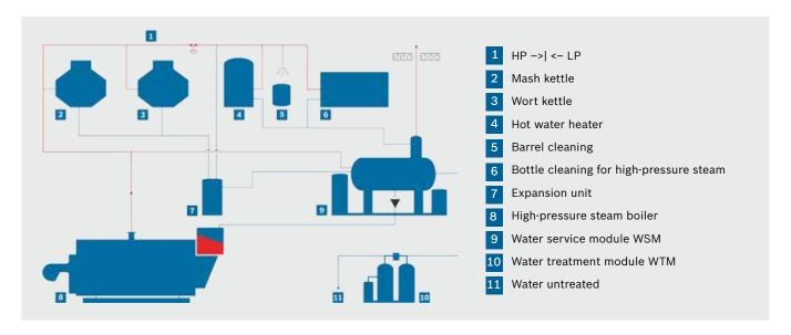
Figure 4: Concepts with partial deaeration using a low-priced expansion unit
