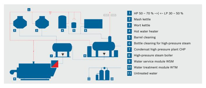
Figure 3: Concept for a partial renewal and use of a HP condensate service module
