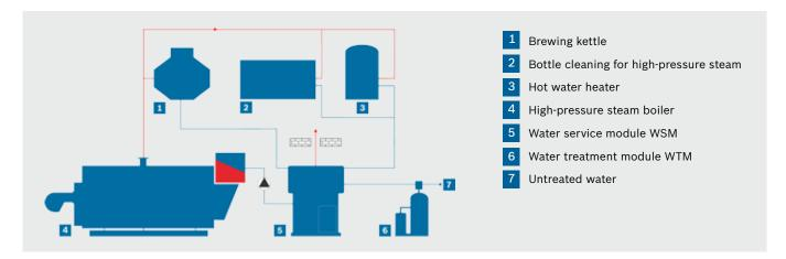
Figure 1: Steam generation for a restaurant brewery with open condensate recirculation
