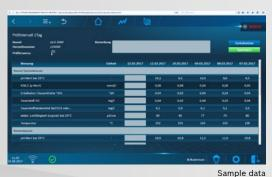
recorded measurement values into the electronic boiler logbook and print these out if required via an export function. The intelligent boiler logbook also checks all entered data, then compares this with the manufacturer's specifications and gives action recommendations if there are any discrepancies
