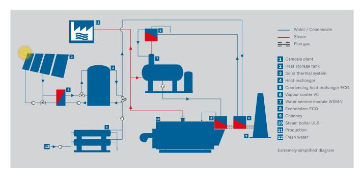
System diagram steam boiler combined with a solar thermal system and heat recovery modules.
