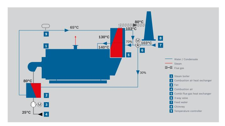
Simplified hydraulic diagram of the Bosch air preheating system at Rauch Fruchtsäfte.
