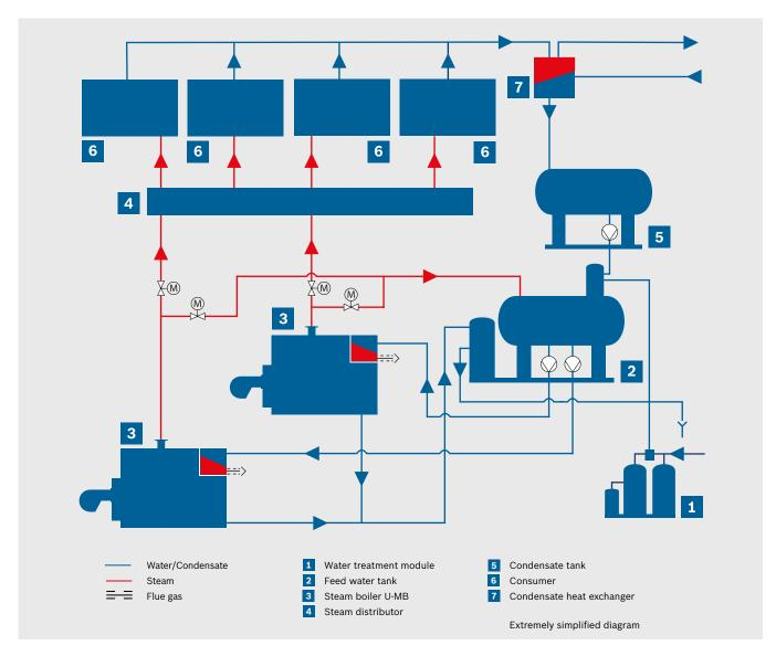
System diagram steam boiler with appropriate plant technology for heat recovery, water treatment and condensate return.
