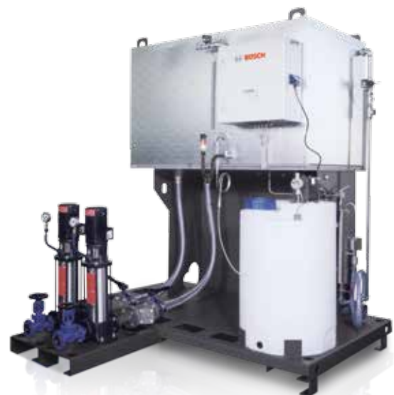
Water service module WSM-V for full deaeration for all steam boilers with outputs ranging from 2,000 to approx. 100,000 kg/h.
