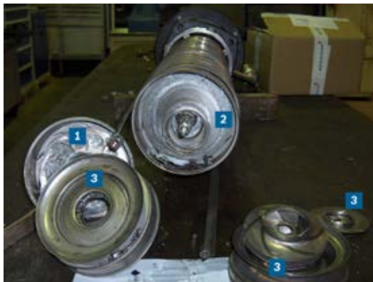
Fig. 26 Pump damage due to cavitation
