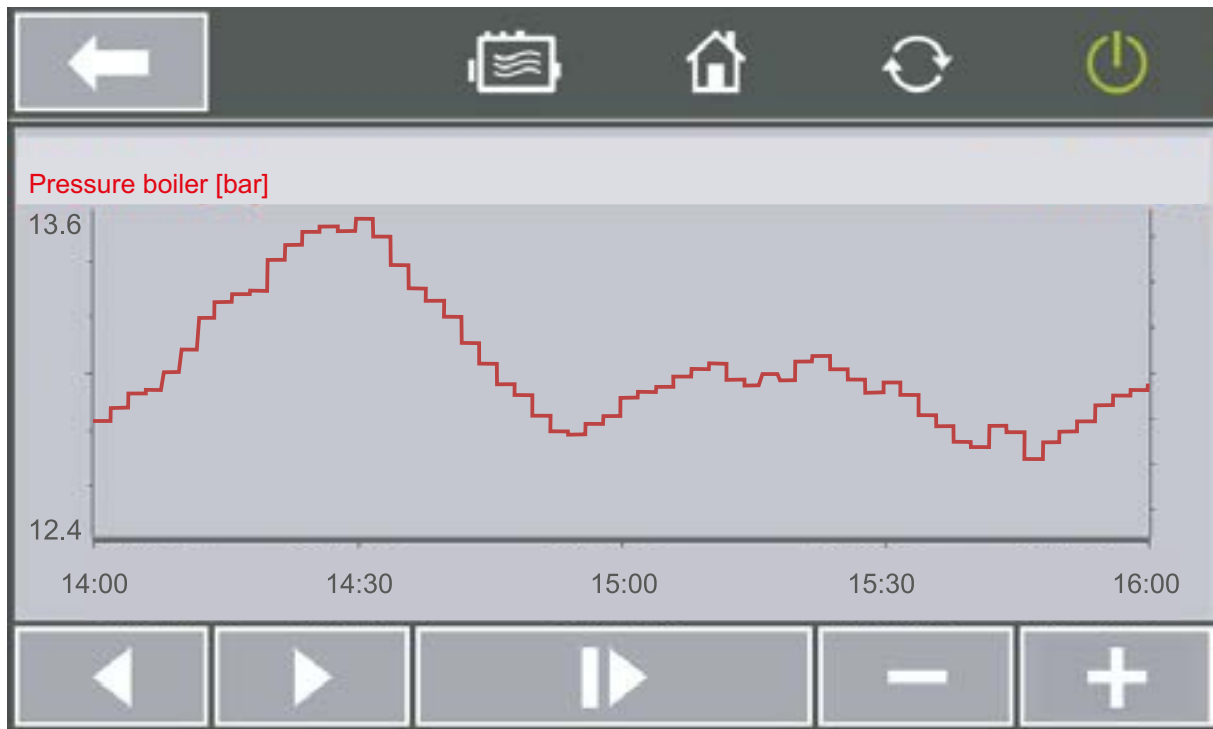
Fig. 5 Illustration of pressure curve over time (boiler control BCO)
