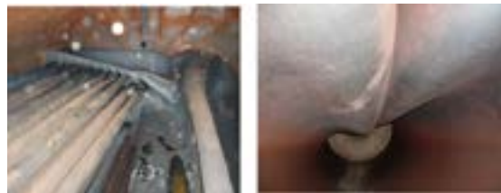
Fig. 33 Deformation due to overheating as a result of water shortage
