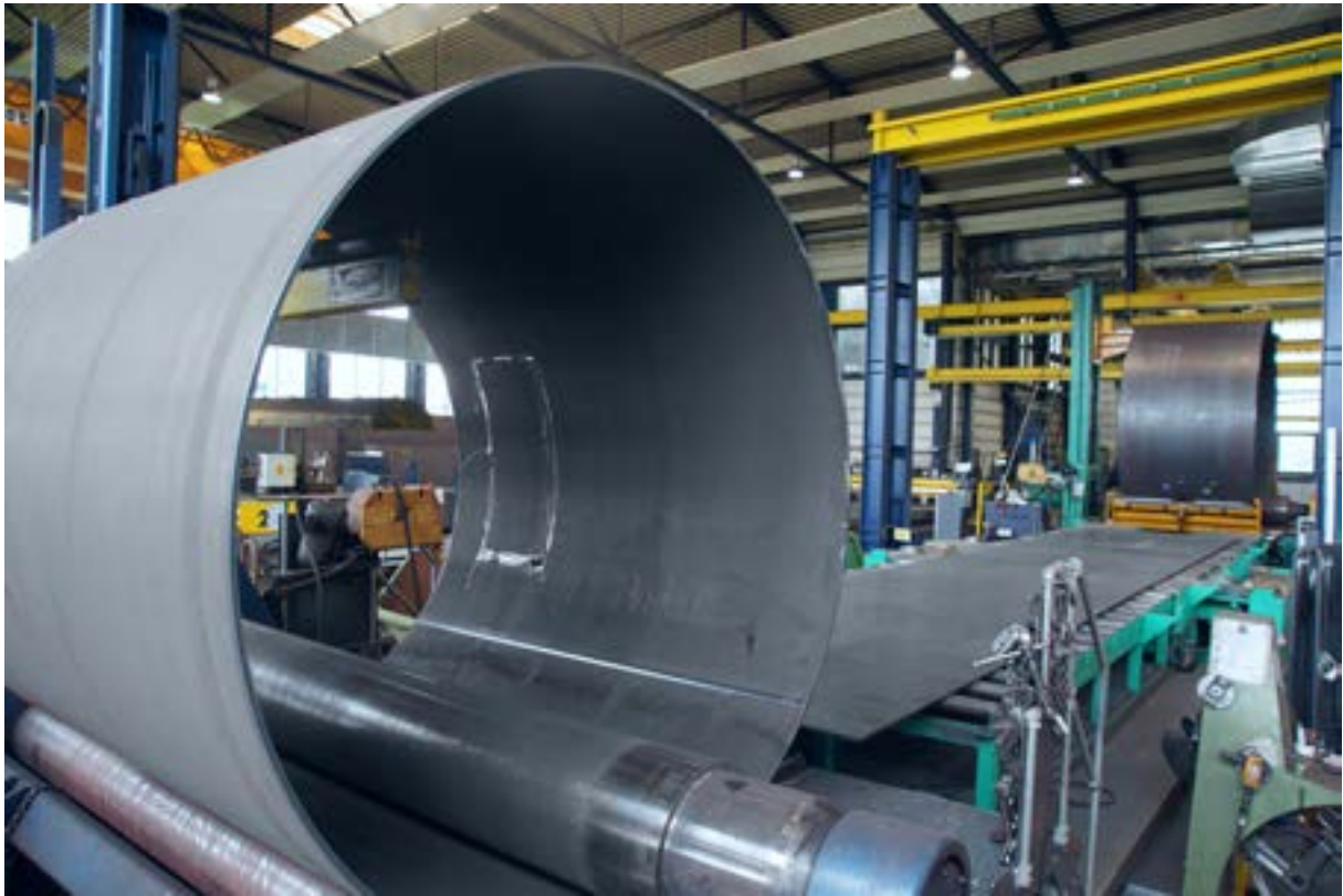
Fig. 133 Bending of sheet metals with widths up to 3.5m is possible
