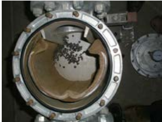
Fig. 31 Welding seam beads and film rust in the gas filter
