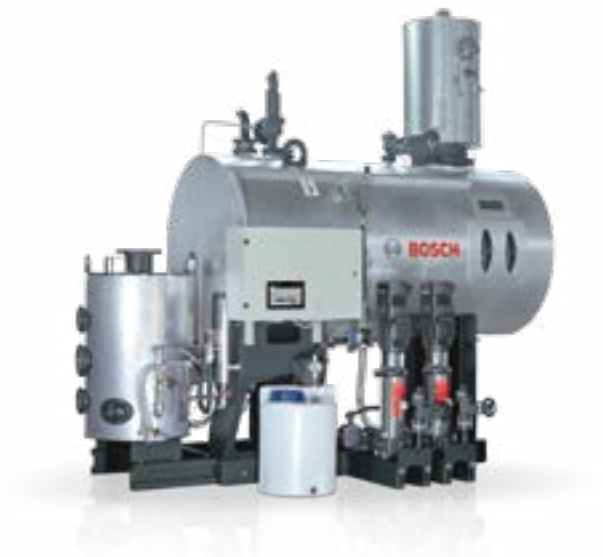
Fig. 97 A water service module, consisting of feed water vessel with trickle deaerator, feed pump modules, blowdown expansion vessel, dosing tanks and corresponding control cabinet
