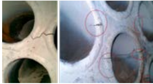
Fig. 24 Flue gas side with cracks in the ribs in the tube plate of the reversing chamber
