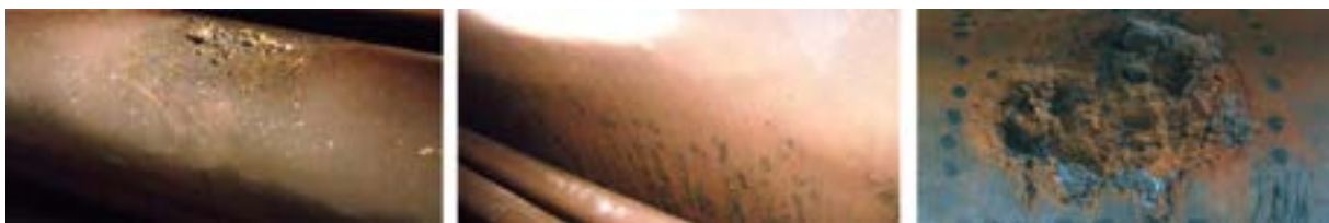
Fig. 95 Damage due to oxidation in the boiler and on the pipework
