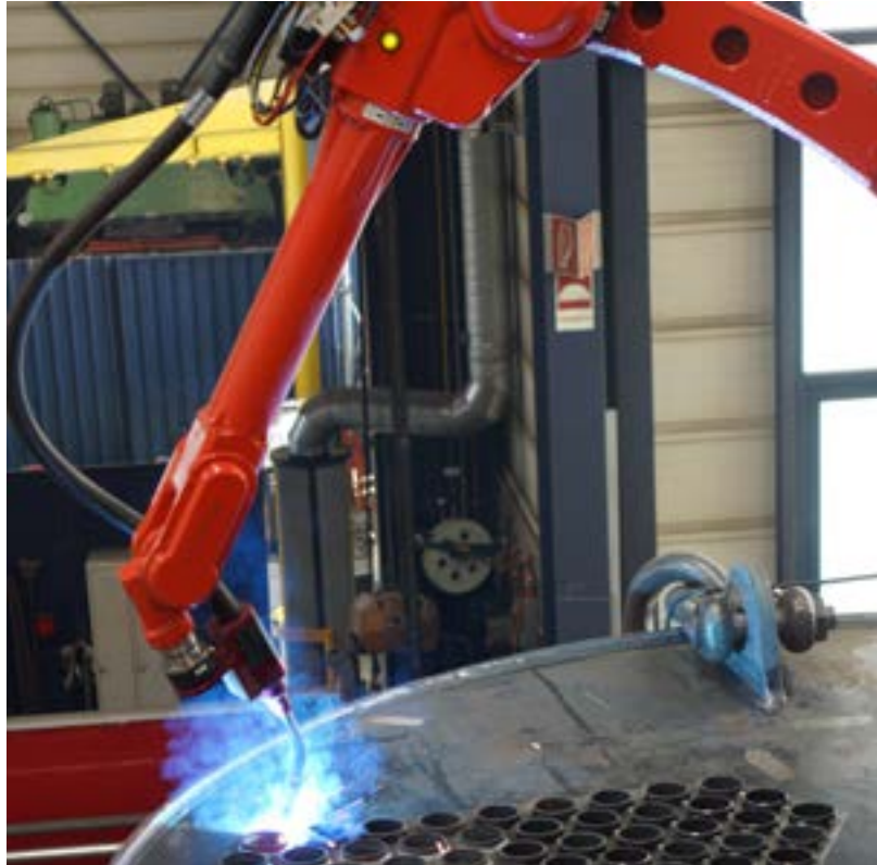
Fig. 132 Mobile welding robot used in Bosch industrial boiler production
