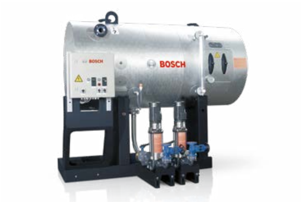
Fig. 201 The unpressurised condensate service module collects the condensate streams and channels them back into the water/steam circuit via the deaeration system
