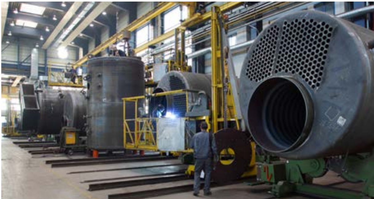
Fig. 130 Horizontal and vertical boiler shells at the production in Gunzenhausen, Germany
