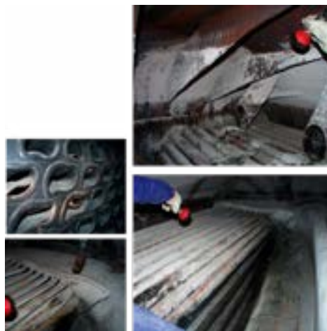
Fig. 25 Layer of grease and contamination in the boiler resulting in deformation of the flame tube and internal reversing chamber due to overheating
