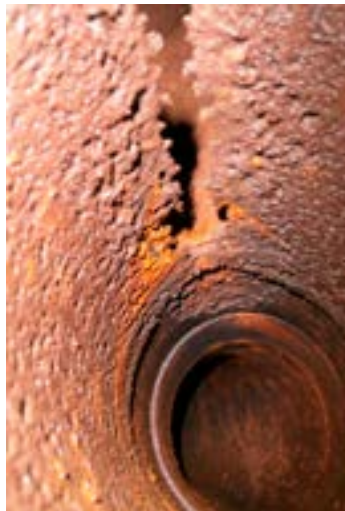
Fig. 15 Introduction of waste water at temperatures over 100°C at the bottom blowdown vessel below the water line (at the connector for <100°C)
