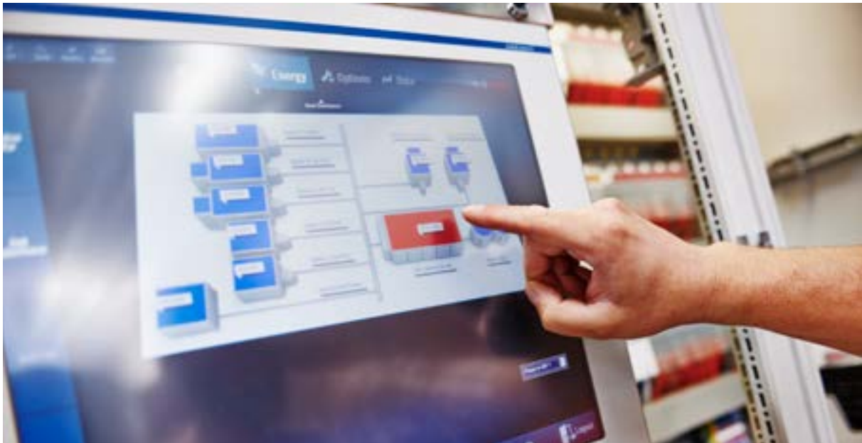
Fig. 226 MEC System for coloured clear visualisation of location and operating conditions, temperatures and performance of systems
