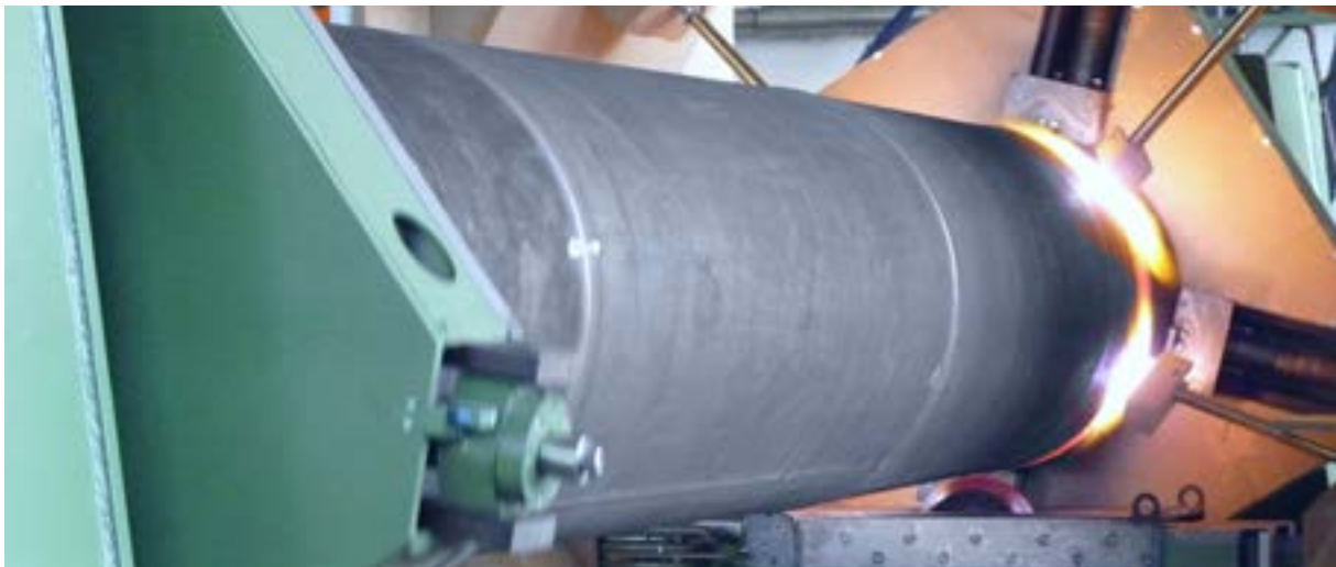
Fig. 131 The in-house designed fully automatic corrugated flame tube machine
