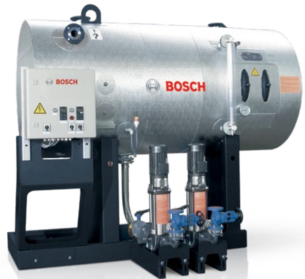
The unpressurised condensate service module collects the condensate streams and channels them back into the water/steam circuit via the deaeration system.
