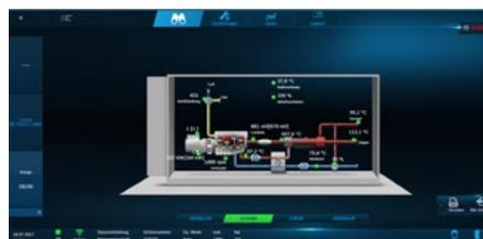
Schematic representation with the most important technical data at a glance. It is possible to switch between different schematic views and levels of detail.
