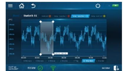
The **statistics display** can be configured as needed, and contains all recorded data points. Individual data can be shown or hidden as required, for additional clarity. Time intervals used in the display can be freely selected.
