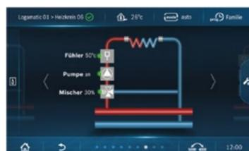
Monitoring/manual control of the heating circuit
