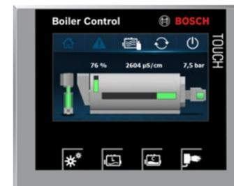
The intuitive visualisation of the CSC on the **overview screen** delivers the status of the burner, boiler and feed water pump components, as well as further information about the system status, fuel and operating mode – all at a single glance. A traffic-light model (green/yellow/orange) is used to signal the different states.
