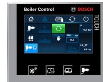
The **burner dialog** offers setting options for burner operation, fuel choice and output regulation. Using the display of the current boiler pressure and the actuating signal for the burner, the working gauge pressure can be set. The output regulation can be operated either manually or automatically.
