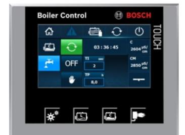
Conductivity control and limits, as well as blow-down, can all be selected to maintain good **water quality** in the boiler. Blow-down can be performed either manually or time-controlled at set intervals.
