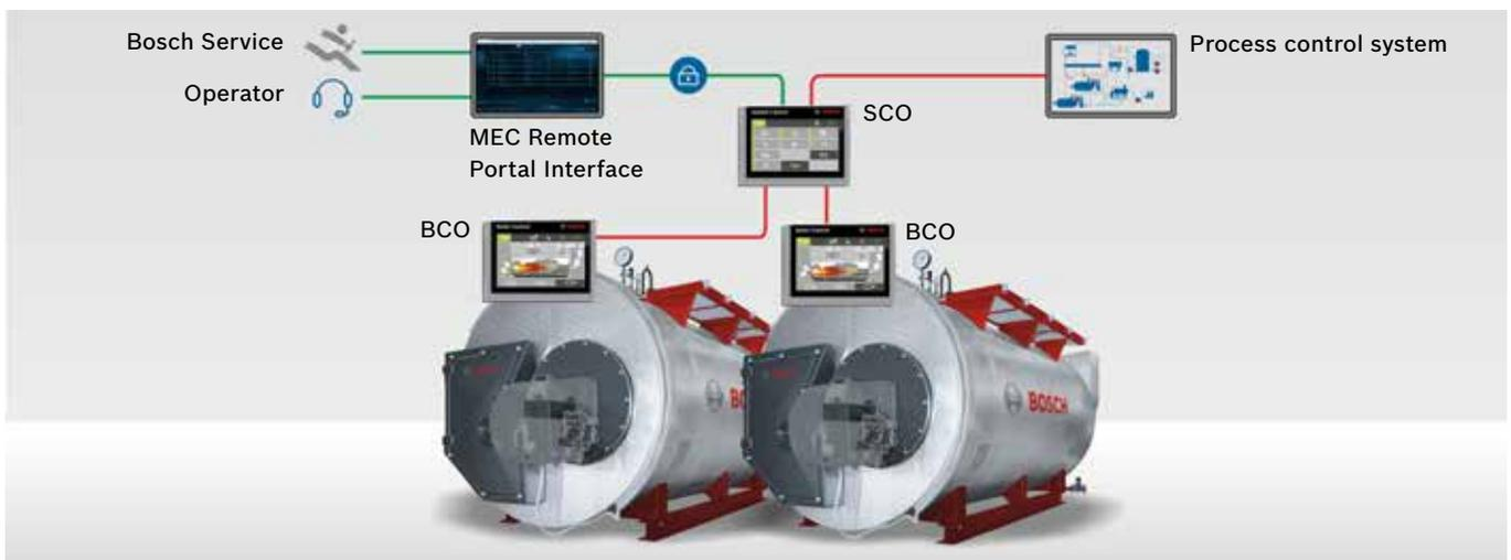
Thanks to an overview map several boilers in different sites all around the world can be monitored at the same time. The optional SMS module sends out defined push notifications whenever an error occurs. This reduces the effort for supervision of plants with especially high reliability requirements, e.g. in 24/7 operation.
