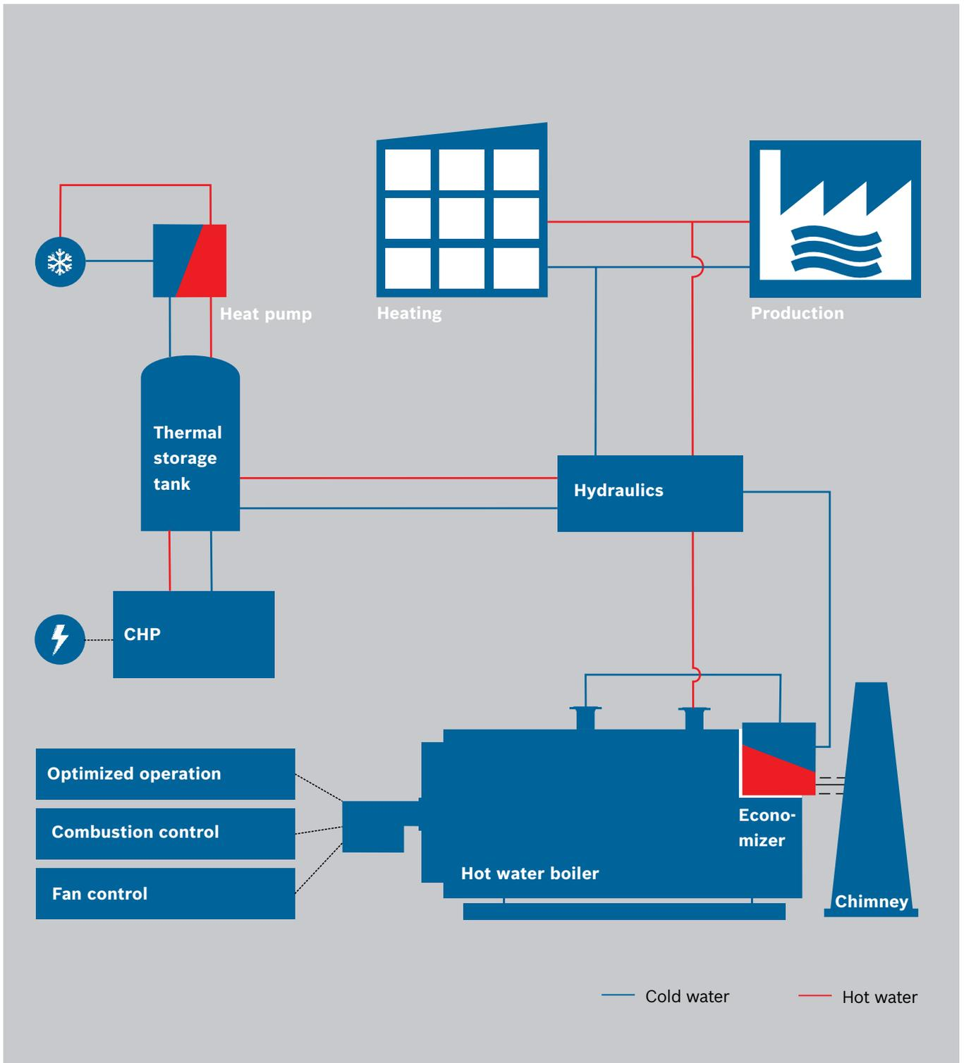
The intelligent combination of energy generation plants into multivalent systems maximises the efficiency and saves resources.
